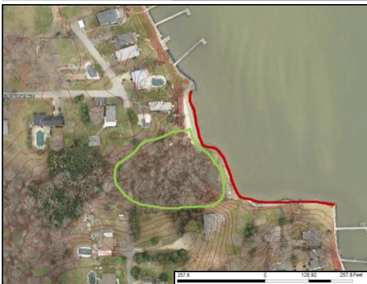
Aerial views of Chesapeake shoreline near Friendship in 1970 (above) and 2015 (below) illustrate the effect of bulk-heading on adjacent shoreline.
